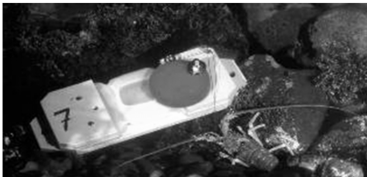
Figure 1: Juvenile lobster attached to a chronographic tethering device for recording time of predation events.
